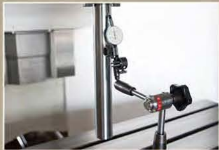
Spindle run-out check
