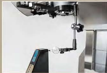
Vertical straightness of Y&Z axis
